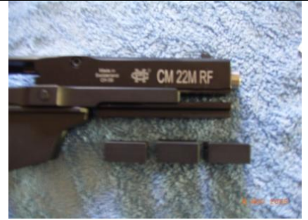
3 Remove barrel weights (makes life easier – you will have to anyway) and cock pistol
