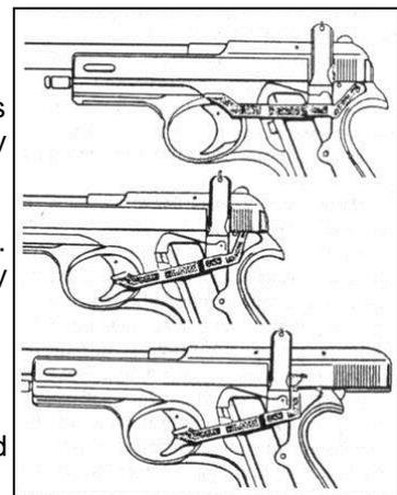
**Removal and replacing the safety catch**
